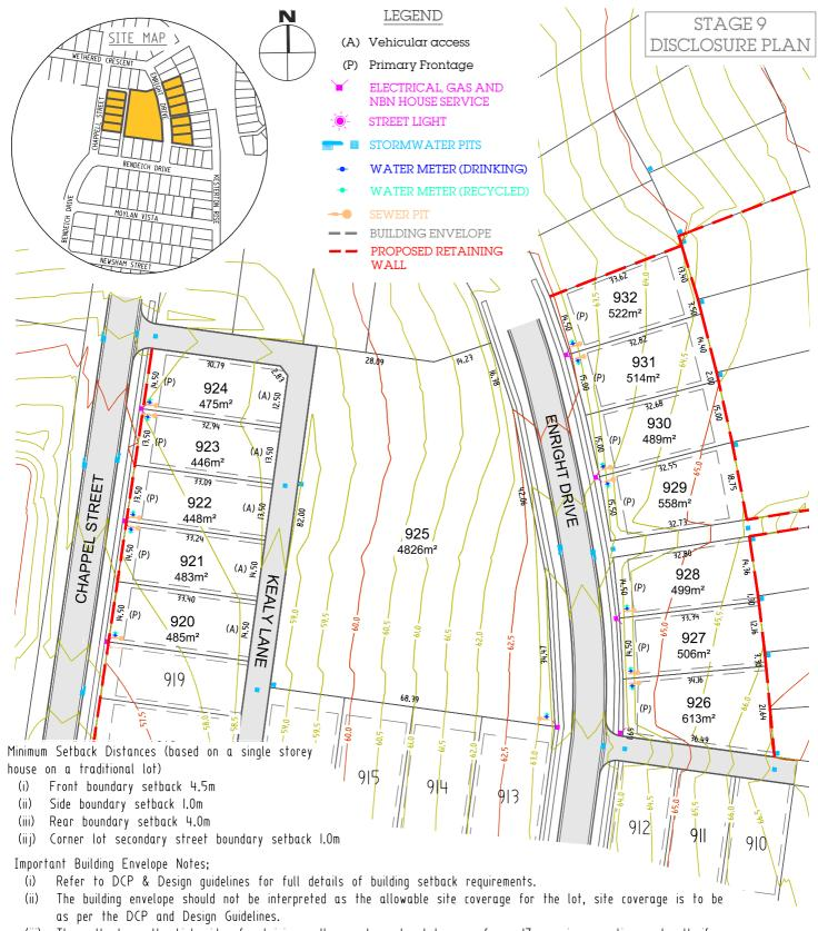
(iii) The setback on the high side of retaining walls can be reduced to zero for a 17m maximum continuous length if the developer provided retaining walls are replaced with a drop edge beam on the house slab (cottage lots only).
